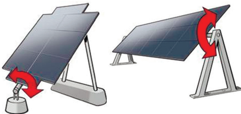
Figure 3 6: Polar and horizontal types of single-axis tracker 1
