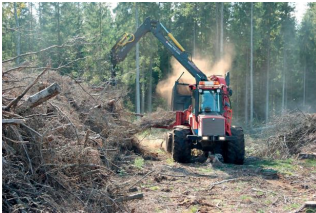
Comminution of logging residues by a truck-mounted chipper
