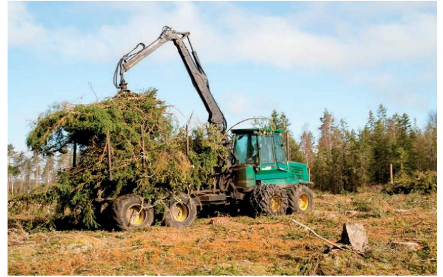
Haulage of logging residues by a forwarder
