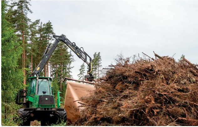
Stacking of logging residues by a forwarder
