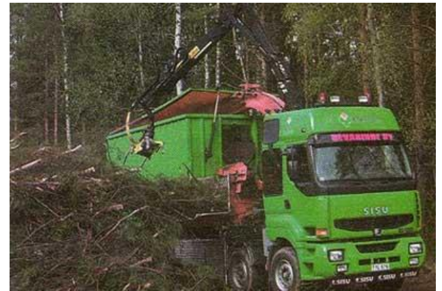
Comminution of logging residues by a chipper-truck
