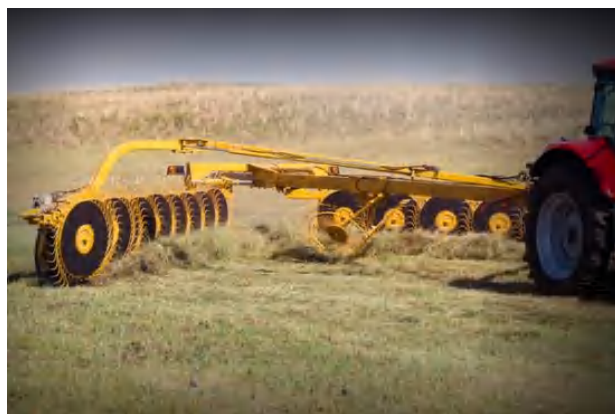
Fig. 25. Biomass windrowing with Vermeer VR2040 rake.
