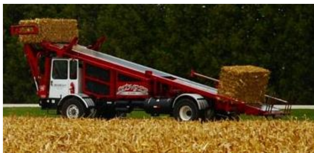
a – truck Stinger Stacker 6500; b – large square bale picker/stacker 16K Plus Bale Runner
