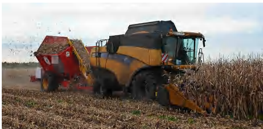
Fig. 27. Grain corn harvester with cobs harvester – COBS HARVESTER Lafargue Bio Energy.
