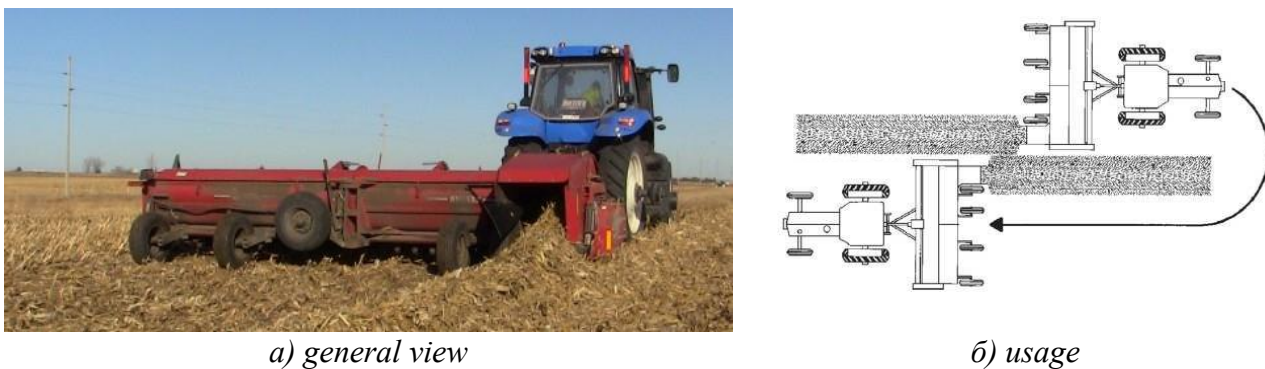
Fig. 21. Machine for crop residues shredding and windrowing Hiniker 5620.
