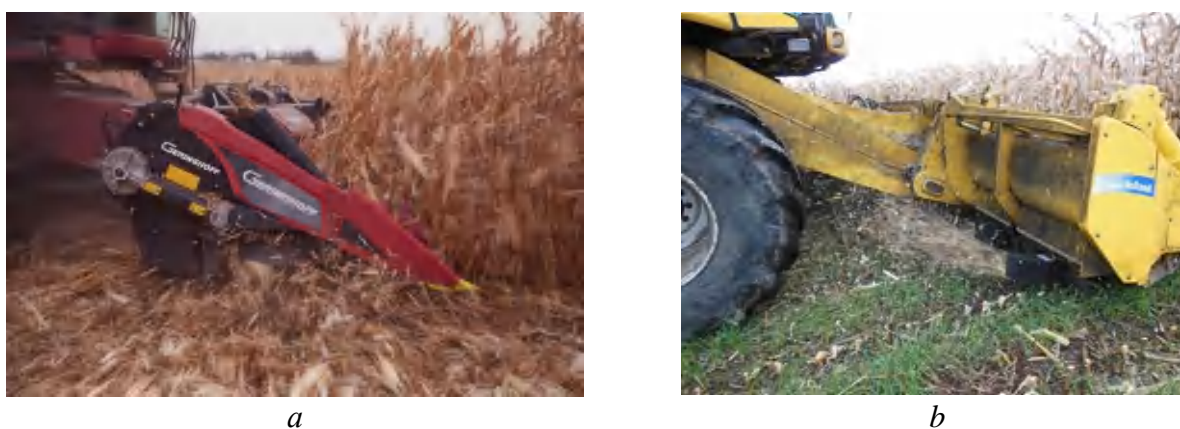
a – Geringhoff Mais Star Collect; b – New Holland's Cornrower
