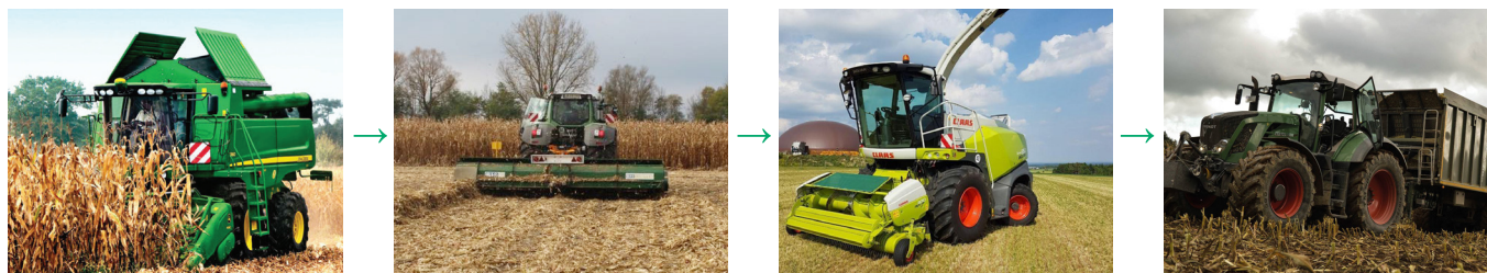
a) Forage harvester system: combine + tractor with stalk-shredding windrower + forage harvester + tractor with trailer
