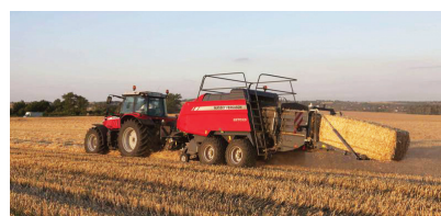
c) Combine + tractor with stalk-shredding windrower + tractor with baler
