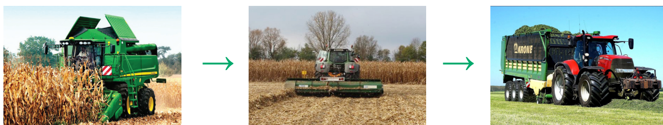
b) Forage loader wagon system: combine + tractor with stalk-shredding windrower + tractor with forage loader wagon
