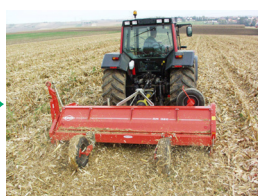
d) Combine + tractor with stalk-shredder + tractor with rake + tractor with baler
