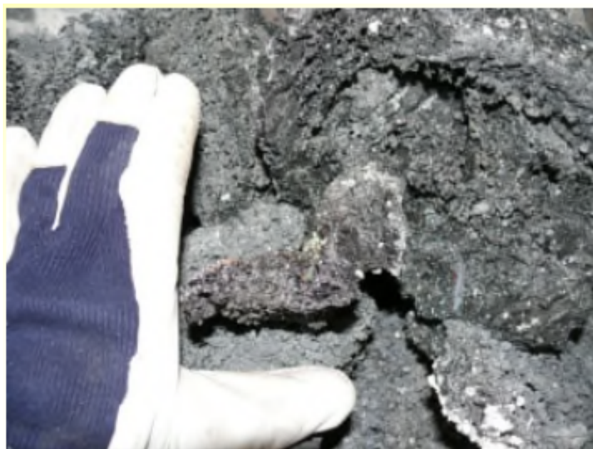
sintering of ash (wheat straw as fuel)
