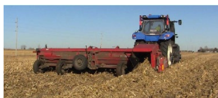
c) Combine + tractor with stalk-shredding windrower + tractor with baler
