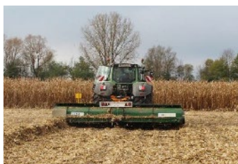
b) Forage loader wagon system: combine + tractor with stalk-shredding windrower + tractor with forage loader wagon
