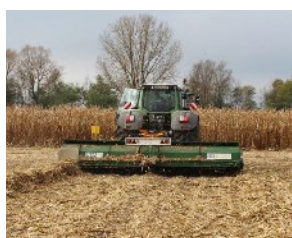
a) Forage harvester system: combine + tractor with stalk-shredding windrower + forage harvester + tractor with trailer
