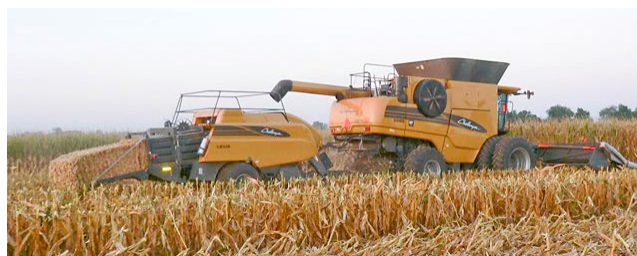
a) Single-pass harvesting system: combine with baler
