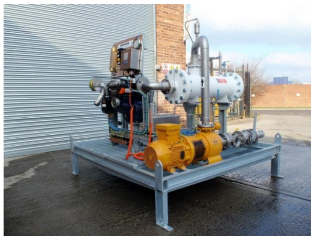
Fig. 2.6. Pumping systems for aviation fuel [46].
