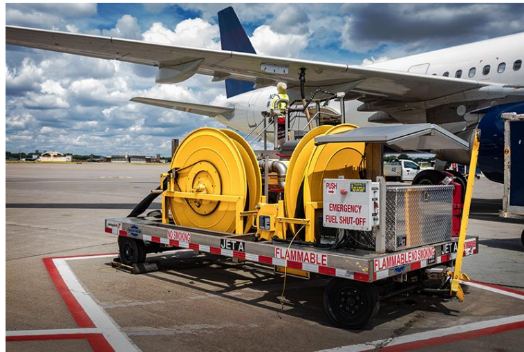
Fig. 2.8. Refueling the aircraft by means of CRA system using: a) a hydrant on the car chassis; b) a hydrant on the cart.
