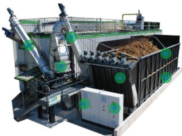
Fig. 5.4 – BIOCRUSHER equipment: a) equipment layout; b) crusher
