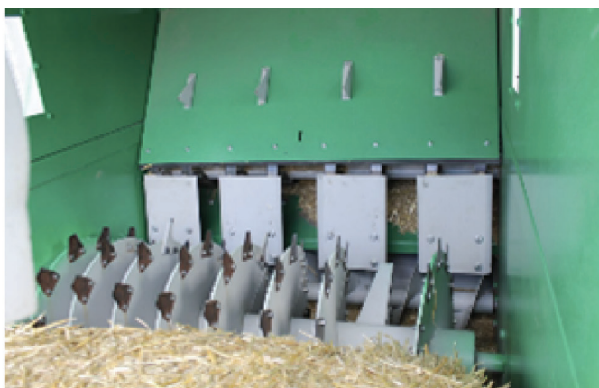
Fig. 9.1 – Straw feeding and pretreatment line (photo by HoSt)
