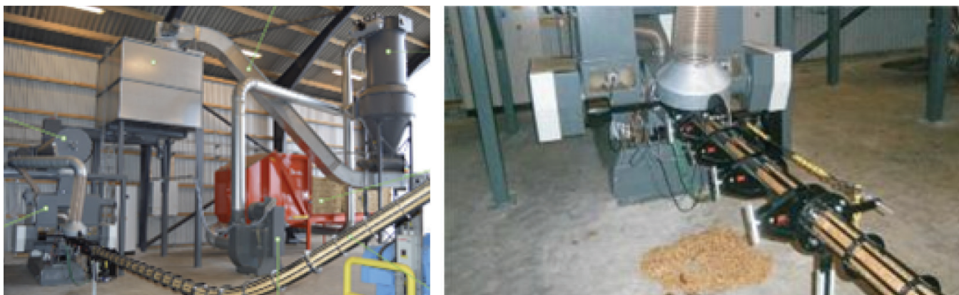
Fig. 9.2 – Straw briquette feeding line
