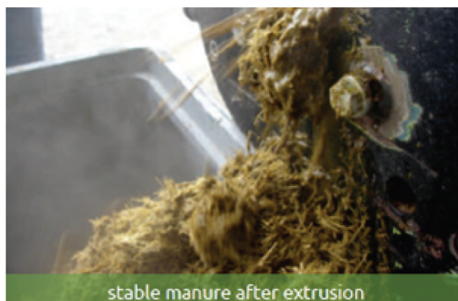
Fig. 5.8 – Cattle manure before and after processing in a bioextruder
