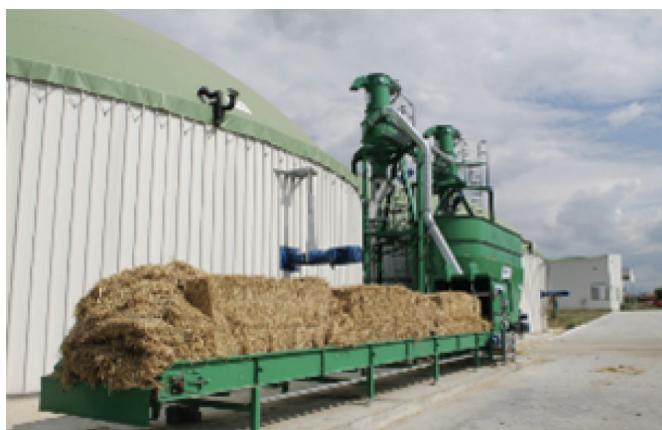
Fig. 9.1 – Straw feeding and pretreatment line (photo by HoSt)
