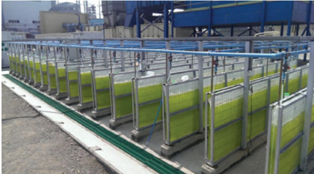
Fig. 2.4 - Pilot flat-panel photobioreactor system (1.5 m height, 10 m length, 0.10 m width), located in Tocopilla, Chile, at the E-CL power station 71
