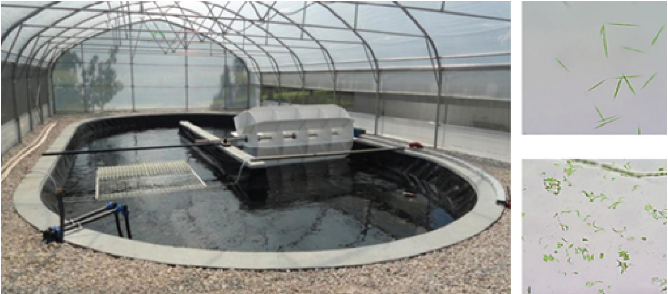
Fig. 7.2 - Photo of the AlgaeBioGas demonstration centre in Slovenia, implemented at an operating biogas plant. On the right, an image of the microalgal consortium from this installation
