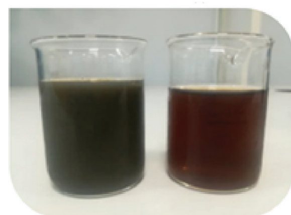
Fig. 4.1 - Digestate before (left) and after (right) microfiltration using a ceramic filter with 0.1 µm pores
