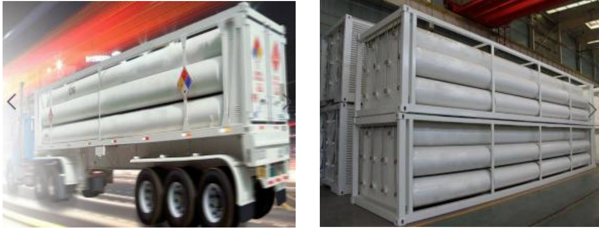
Fig. 3.5. Containers for storage and transportation of compressed natural gas 80
