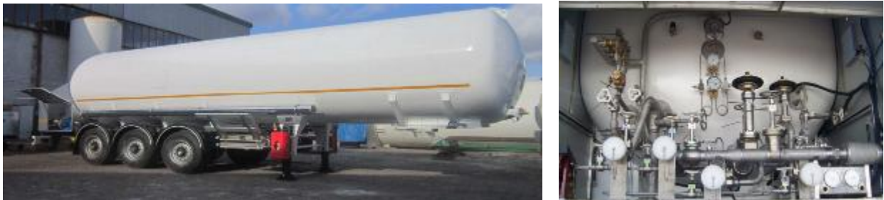
Fig. 3.10. Tanker-semi-trailer for transportation of bio-LNG.
